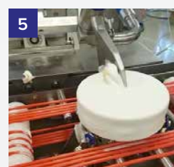
Cream and icing side and top masking station
