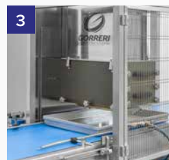
Cream filling station with manifold
