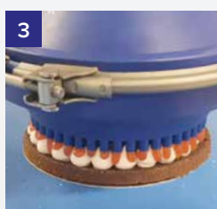
Jam filling dosing station
